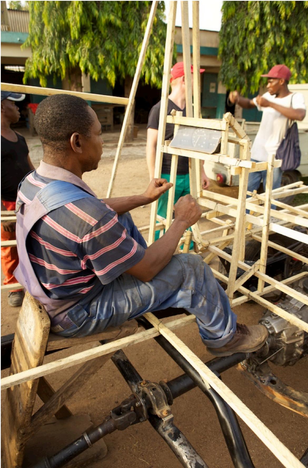
Building the 1:1 wooden test model of Turtle 1 © Teun Vonk
